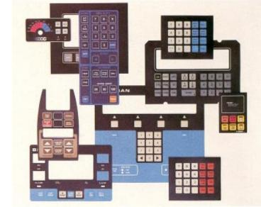
Substrate Material. All MSI *Microterm*™ keyboards are fabricated on glass-epoxe substrates and feature gold plating (over nickle underplate) for all switch-related circuitry.
